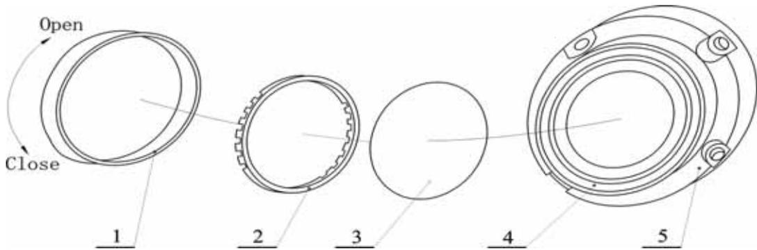
1. Gland of filter; 2. Rubber gasket; 3. Filter paper; 4. O-ring; 5. Filter body
