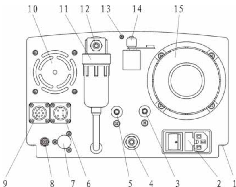
1. Fastening bolt on base plate; 2. Power socket and switch; 3. Gas outlet of O<sub>2</sub> sensor;
