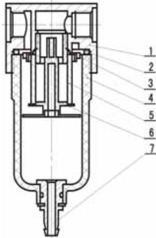
1. Body; 2. O-ring; 3. Cyclone blades; 4. Water-separating cup; 5. Filter core;
