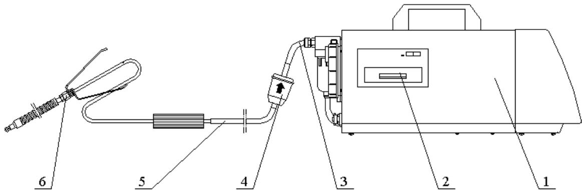
1. Instrument body; 2. Micro printer; 3. Short tube; 4. pre-filter;
